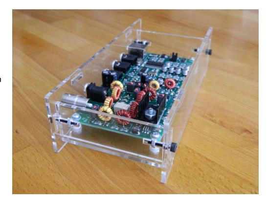
With all the panels installed you can tighten the M3 hardware with the included wrench. Insert the long end of the wench into the screw caps so you do not overtighten these.
