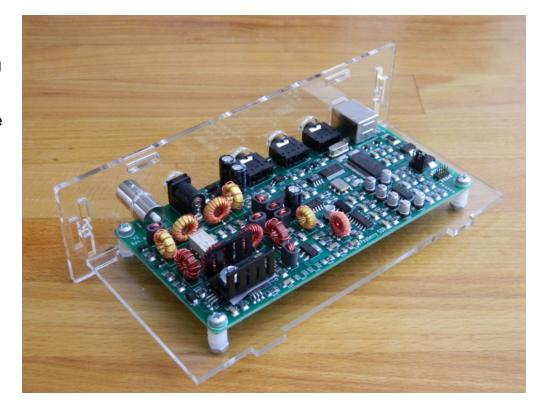
Install the inner side panels and the M3 hardware. Hold the nuts in place with your fingers when starting the screw. Install the screws only finger-tight for now.
