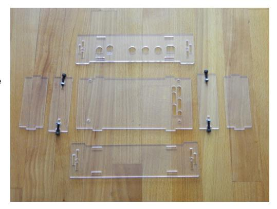
Begin by attaching the circuit board to the bottom panel. The 1/2" #4 screws that came with your radio aren't long enough so use the 5/8" #4 screws that came with the case. The case also comes with four more nylon washers to put between the nut and the acrylic.
